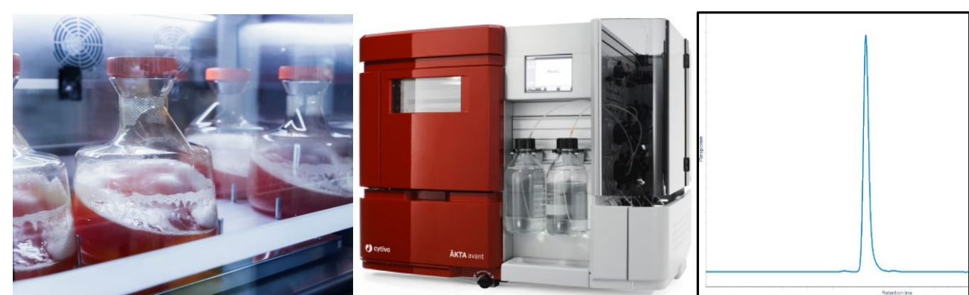
Figure 2. Stable Pool Material Generation (≥ 10 g for standard mAbs). Purified using state-of-the-art ÄKTA™ systems yielding ≥ 95% purity and low endotoxin.
