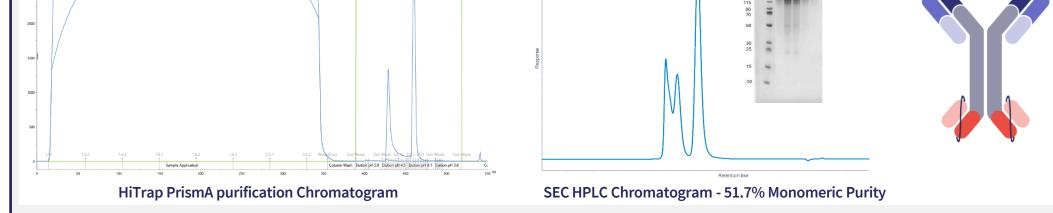
Standard Protein A affinity chromatography capture with step pH elution led to low product purity with high levels of HMWS, possibly a consequence of the scFv.
