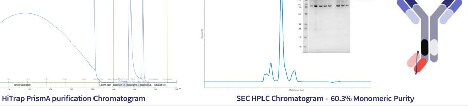
Standard Protein A affinity chromatography using step pH elutions led to different profiles being observed. As anticipated, a milder elution resulted in increased proportion of bispecific compared to homodimer, whereas harsher elution favoured the homodimer.
